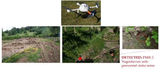
Figure 7. Detection of mines and UXOs after heavy floodsin Bosnia Herzegovina (2014)
